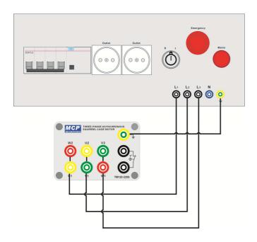
When the motor is connected as above, the motor is normally running.
