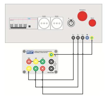
When the motor is connected as above, the motor is running as reduction voltage starting. This connection is just for reduction current. But at this connection, the output power is smaller than 120W. (The power supply's model number is TB412.)
