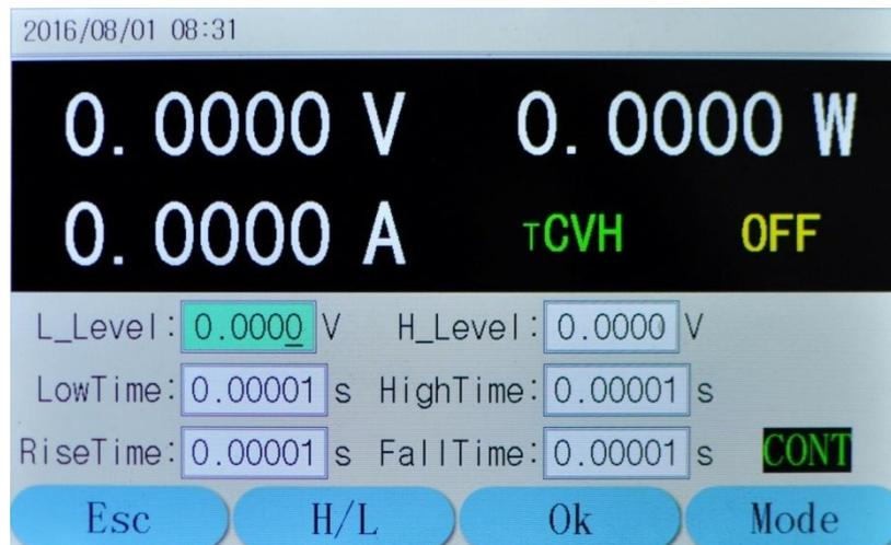
**Step 2:** Select “L\_Level” via **Tab** key or **▲** and **▼** keys; enter the transient low level 10 by the number keypad, or via knob with **◀** and **▶** keys; then press **Enter** key to confirm;
