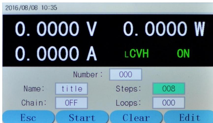
**Step 2:** Set the sequence **Number** to 0 via the keypad or via the knob and then press **Enter** key to confirm;
