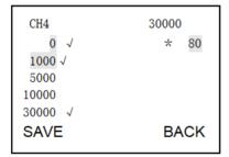
(4) In selecting interface, choose the gas type by pressing (\*\*). Choose the detecting range by pressing "Zero" button. Then press
