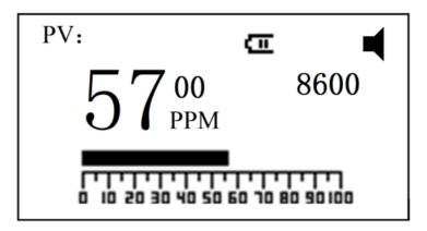
Processing bar --- Proportion of detected gas vs full detecting range.
