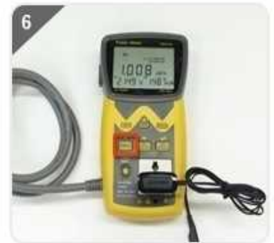
6 After wattage integration press DISPLAY button and change to CO 2 emission mode.
