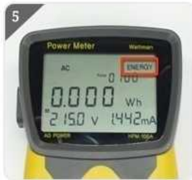
5 "Energy" sign is displayed at the above right of LCD screen and start integration.
