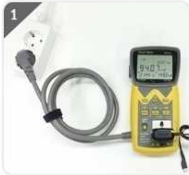
1 Put the plug of measured product in multi-outlet at the below right below of the product after power in.
