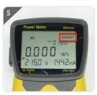
"Energy" sign is displayed at the above right of LCD screen and start integration.
