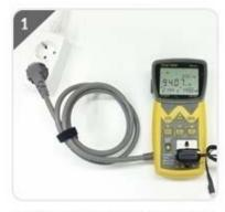
Put the plug of measured product in multi-outlet at the below right below of the product after power in.
