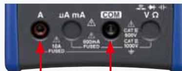
For the 'A' range,\* only the 'A' and COM terminals are accessible; and for the  $\mu\text{A}/\text{mA}$  ranges, only the  $\mu\text{A}/\text{mA}$  and COM terminals are accessible.
