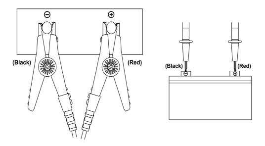
9. Read the battery internal impedance or DC voltage directly and Temperature measurement(TM-6002) from the display.
