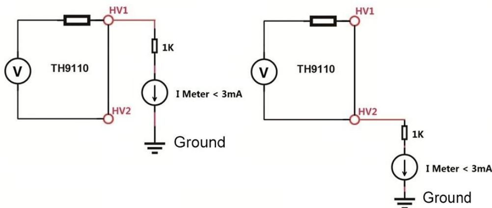
Figure 4-7 Relationship of HV1/HV2 Terminal to the Ground
