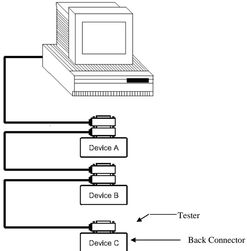
Figure5-2 Double Back Connector Staking
