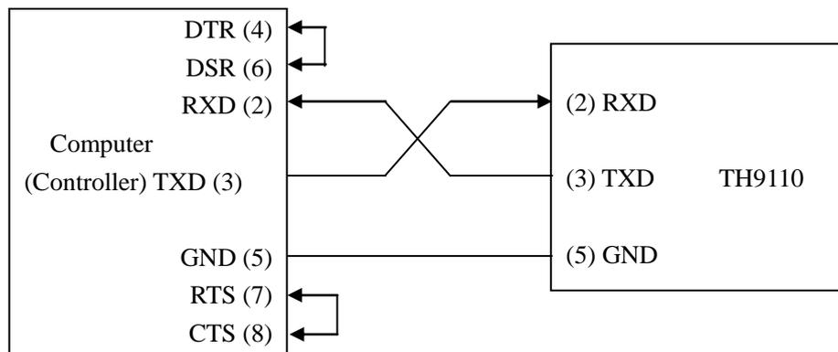
As can be seen from the above figure, the pin definition of this tester is the same as that of the 9-core connector serial interface pin used by the IMB AT compatible machine. Users can use the double-core shielded cable to make three-wire connection cable according to the diagram (the length should be less than 1.5m) or purchase the serial interface cable between the computer and the instrument from our company or directly purchase the standard DB9 core cable (cross line).
