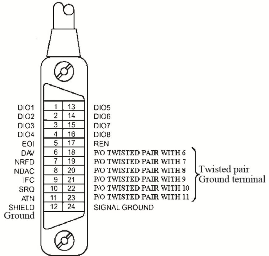
Figure5-1 GPIB Connector/Pin Structure Diagram
