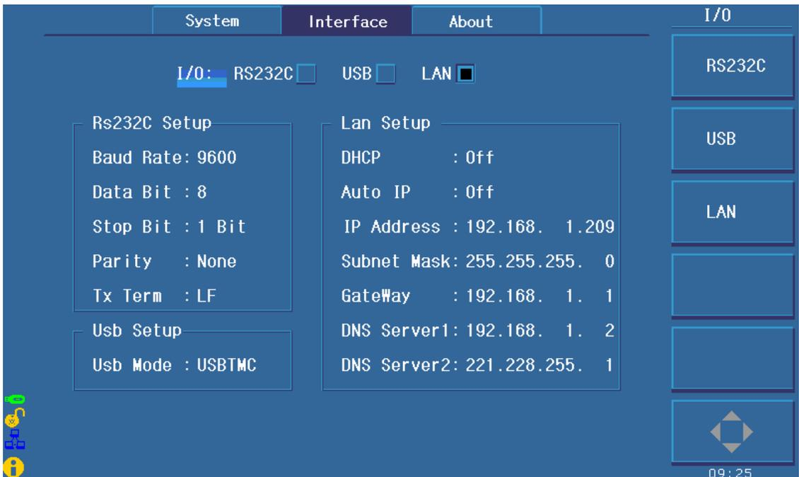
Figure 6-9 Network parameters of TH2883
