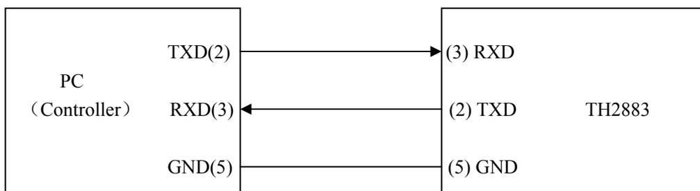
**Figure 6-3 Connection of the instrument with PC**
