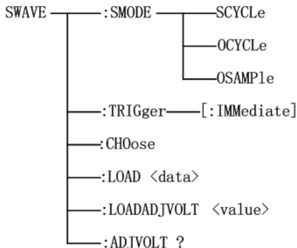
Figure 8-9 Standard WAVE subsystem command tree
