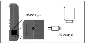
Figure 7-Connecting AC Adapter to Meter
