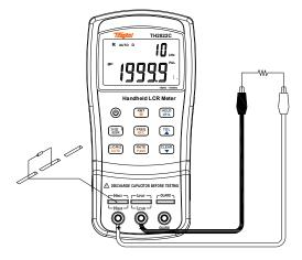
Figure 15- Resistance Measurement
