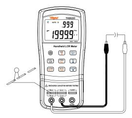
Figure 14- Capacitance Measurement
