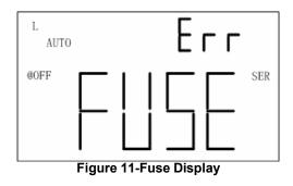
In the event that the above screen is displayed, the instrument should be powered off. If this does not power off the meter, remove external AC adapter if that is used and/or remove the battery from the battery compartment. Please contact after-sale department of our company or appointed distributor for the change of fuse or maintenance. **NOTE:** Both fuse damage and none output of test signal caused by signal source fault will make "FUSE" alarm.
