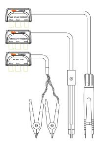
Figure 13- 4-terminal Test Accessories
