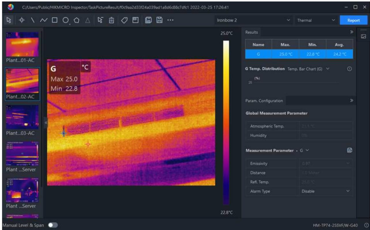
Figure 5-6 Analysis in HIKMICRO Analyzer
