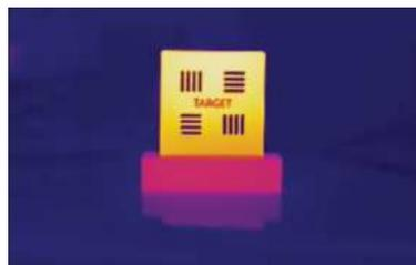
7. Adjust the target's optical image with navigation buttons until it overlaps with the thermal image, and press
