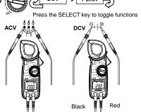
If the connection is reversed, the LCD indicates the ‰ %mark (DCV
