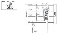
Press the item switching button [▶] after making connection, the LCD shows active power of R(L1) phase. Pressing mode button switches the indication between active power of R(L1) phase and RMS voltage/ current values.
