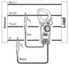
Another press of item switching button [▶] changes measurement object from S(L2) to T(L3).
