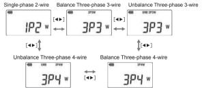
Press the mode button while the desired wiring configuration is displayed. The selection is confirmed and the display returns to the selection screen.
