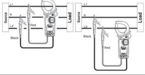
Connection diagram for balance Three-phase 3-wire (3P3W)
