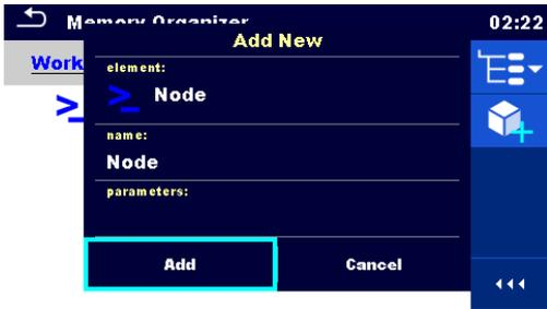
Change name of the Node if necessary and press Add to confirm.
