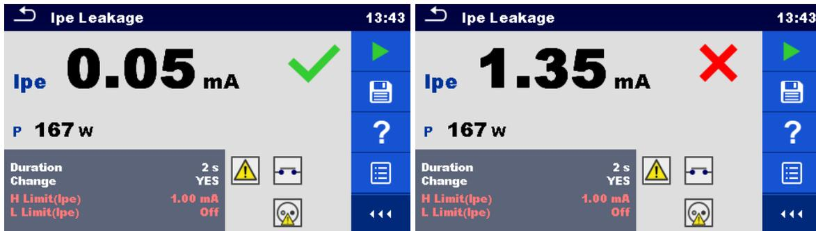
Figure 6.42: Examples of Ipe Leakage measurement results
