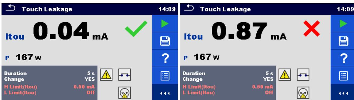
**Figure 6.45: Examples of Touch Leakage measurement results**
