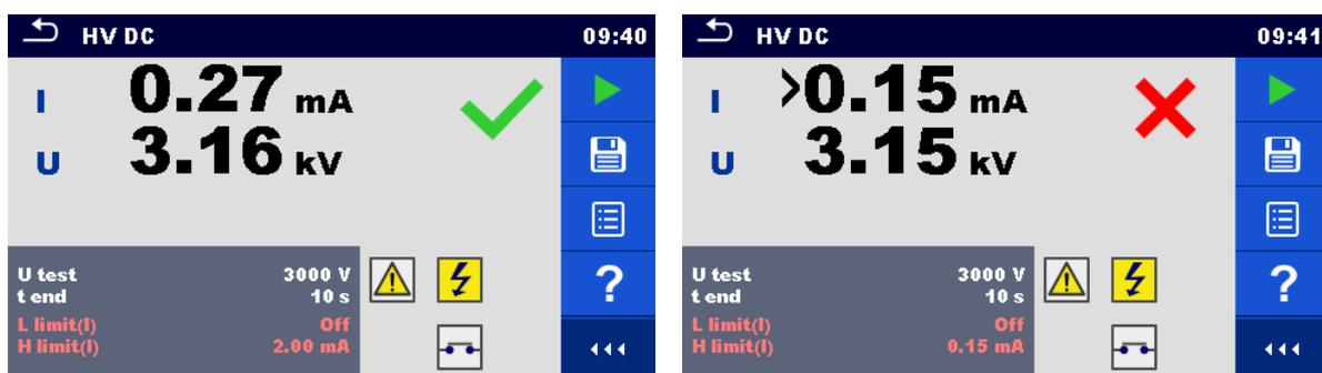
Figure 6.19: Examples of HV DC measurement results
