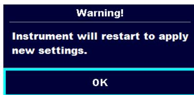
Warning for restart of the instrument to set new Ethernet settings. This message appears on exit from Settings menu after changing Ethernet settings.
