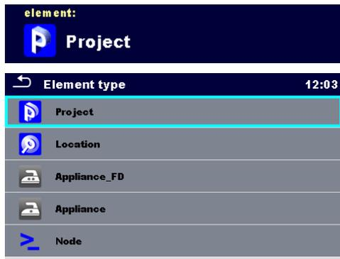
The type of Structure object to be added can be selected from dropdown menu.
