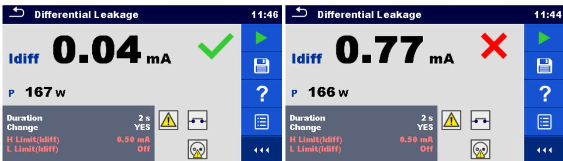
Figure 6.39: Examples of Differential Leakage measurement results
