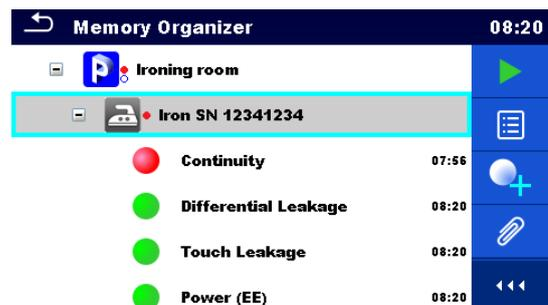
**Figure 5.6: Status - Measurements completed with fail result(s)**
