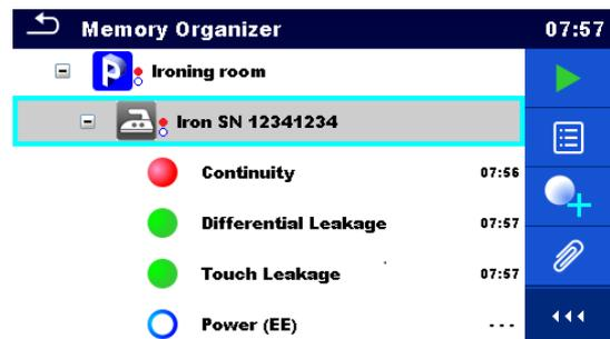
**Figure 5.5: Example of status - Measurements not completed with fail result(s)**
