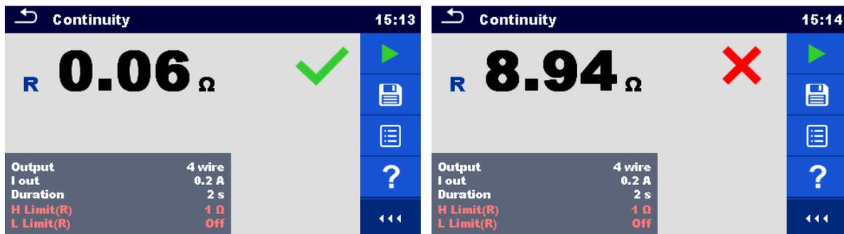
Figure 6.11: Examples of Continuity measurement results
