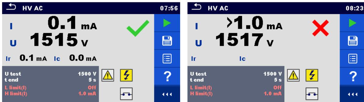
Figure 6.16: Examples of HV AC measurement results
