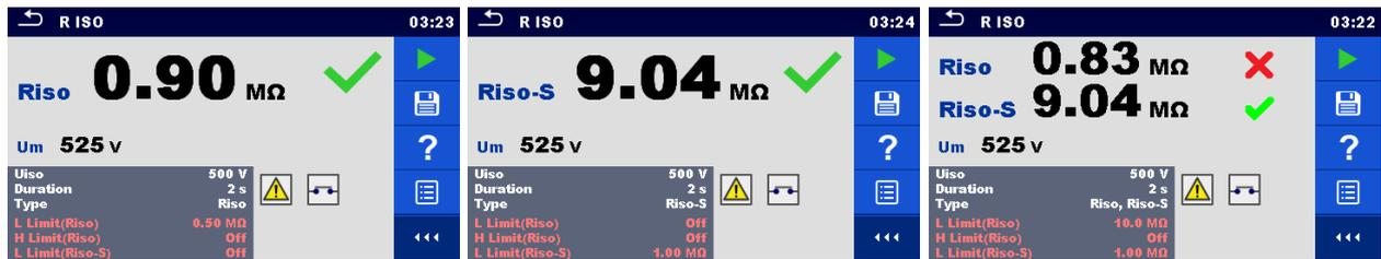
Figure 6.31: Examples of Insulation resistance measurement results
