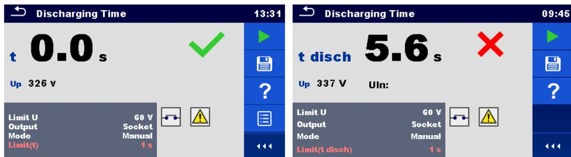
Figure 6.57: Examples of Discharging Time measurement results (Output = Socket)
