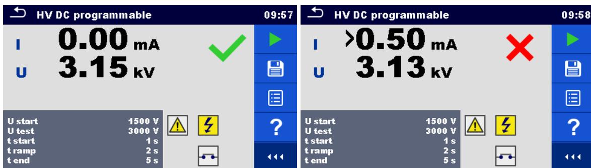
Figure 6.26: Examples of HV DC programmable test results
