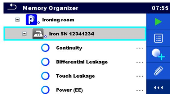
**Figure 5.4: Example of status - No measurement result(s)**
