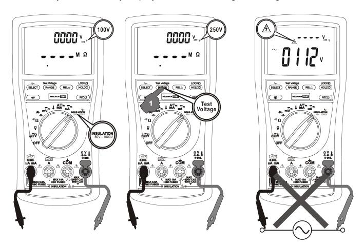
The **TEST** is active as long as the **TEST** button is pressed and hold. The **TEST** buttons on the meter and on the Remote Probe work alike. The Insulation Resistance readings are shown on the primary display.
