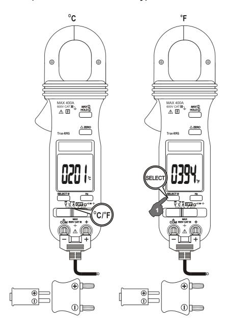
Be sure to insert the banana plug type-K temperature bead probe Bkp60 with correct + polarities. Slide-switch on defaults at degree C (Celsius). Press **SELECT** button momentarily to select degree F (Fahrenheit). You can also use a plug adapter Bkb32 (Optional purchase) with banana pins to type-K socket to adapt other type-K standard mini plug temperature probes.
