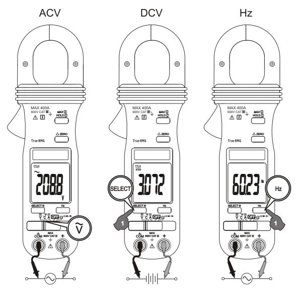
Set slide-switch to Voltage function position. Inputs are made through the test leads terminals. For Models 063s & 065s, slide-switch on defaults at AC voltage. Press **SELECT** button momentarily to select DC voltage. For Models 061s & 062s, separate ACV & DCV slide-switch positions are being used.
