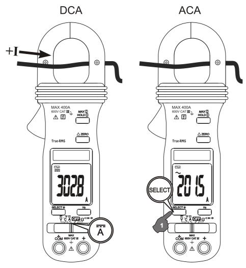
Inputs are made through the clamp jaws for non-invasive ACA & DCA current measurements.
